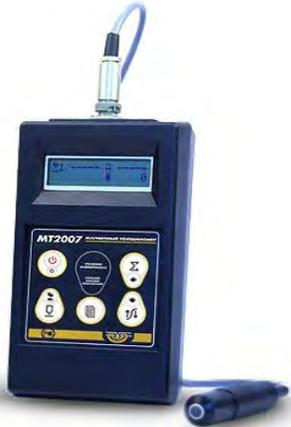
A blue digital coating thickness gauge (MT-2007) with a small LCD screen and several control buttons. A blue probe is attached to the top, and a blue pen-like tool is lying next to it.                                     |
