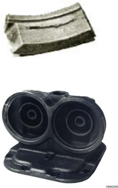
Figure 3-59. Magnetic Particle Indications of Defects in Castings
