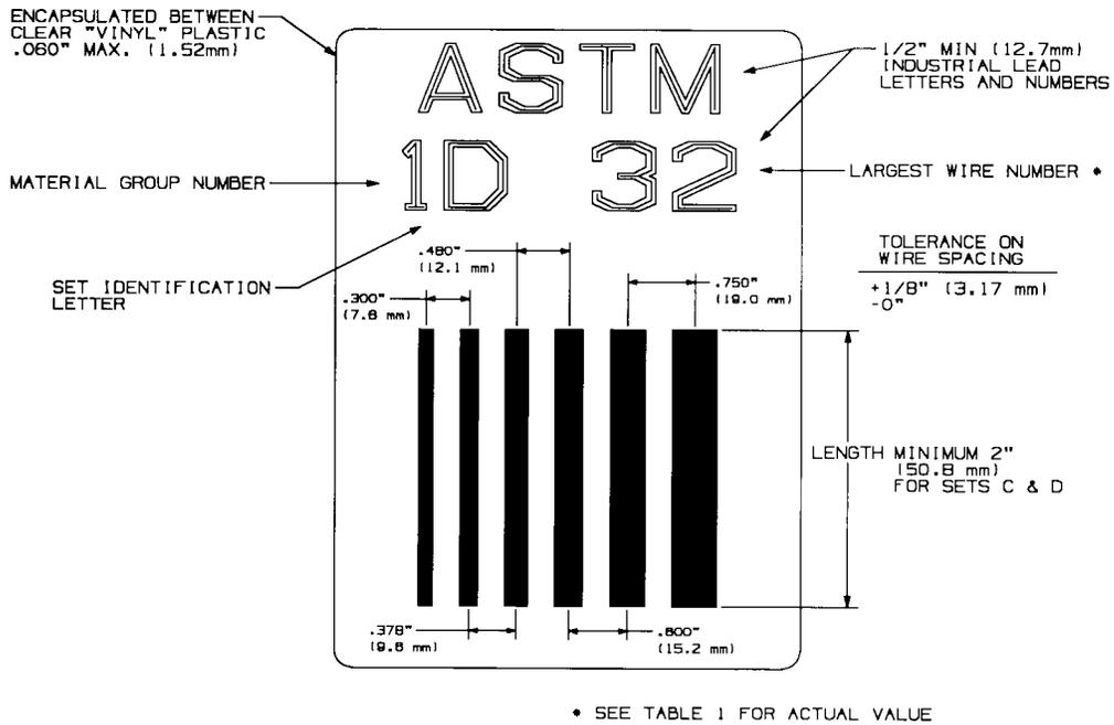
FIG. A1.8 Set D/Alternate 2
